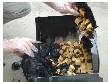
Figure-12 Pail face removed and pail cut open showing intumescent char plug and undegraded FR-3718 foam cubes
